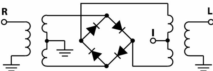
Some local oscillator energy appears at the input of the transformer, but is anti-phase and cancels. For example, a voltage on terminal "L" is induced into the windings either side of terminal "I", but they are of opposite polarity and cancel out.
