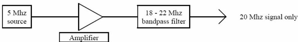
In the above example, a 5 Mhz signal is over-driven. Outputs will be present at 5 Mhz, 10 Mhz, 15 Mhz, 20 Mhz, 25 Mhz, and so on. If a filter that only passes 18 to 22 Mhz is placed on the output, only the 20 Mhz signal passes through. We now have an output that is quadruple the input frequency.
