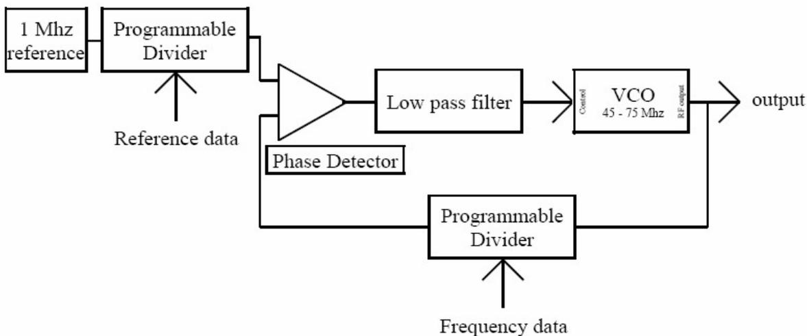
The second divider has now been added. The two are loaded with data that would give the desired frequency of operation, for example:
