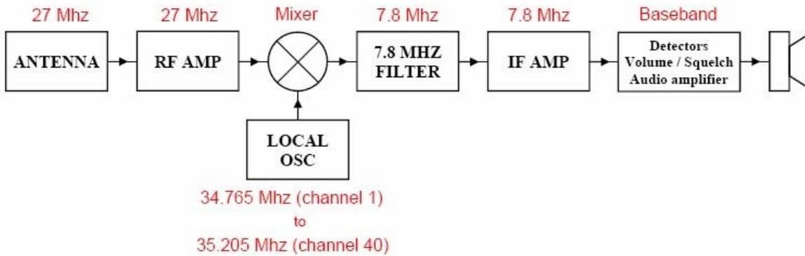
The antenna receives signals on all channels. This mixture of signals is passed through an RF amplifier and then to one input of a mixer.
