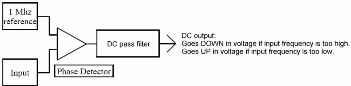
The first (top in this example) is a constant input and never changes - in this case, it's a constant 1Mhz signal from a crystal oscillator.
