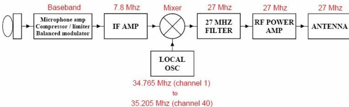
Microphone audio is filtered, compressed, and limited to optimize it for speech and keep the radio within legal limits set by the FCC. This is done at baseband, which is the same frequency as what comes out of our mouths when we talk.
