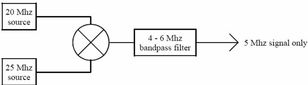
Only one of the 4 will be the desired frequency. A filter always follows a mixer, this will allow the wanted signal to pass through and the other unwanted signals to be rejected. In the above example, only the 5 Mhz signal was wanted, and the passband of the filter was chosen to accomplish this.
