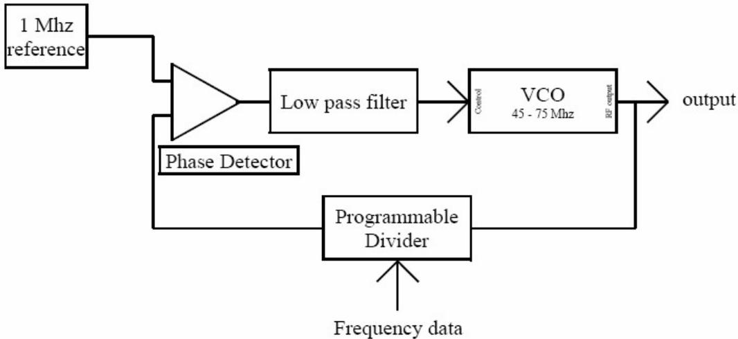
A "Programmable divider" is now added to the circuit. The VCO has also been changed, to one that can change from 45 to 75 Mhz for its 0V to 5V control range - at 2.5V, it would be at its halfway point of 60 Mhz.
