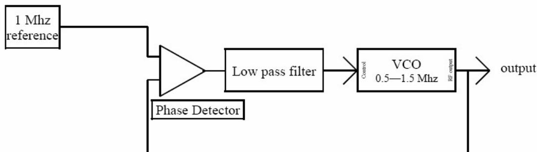
Two circuit sections from the previous sections have now been combined into one unit. Note that a sample of the VCO's output is fed back into the phase detector as the "second frequency".
