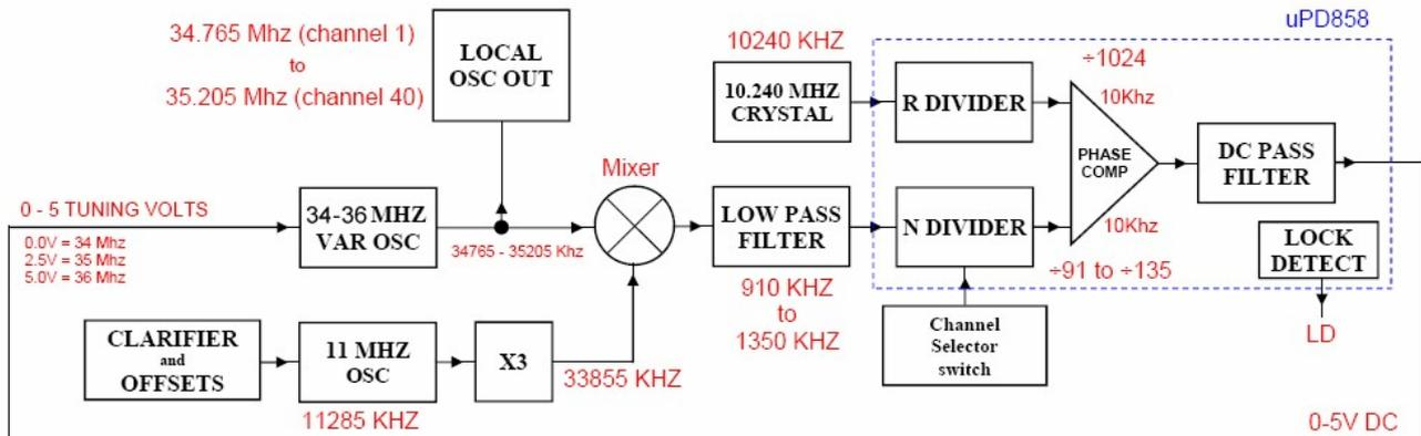
The diagram shows the frequencies present in AM receive mode on the 858 SSB chassis.
